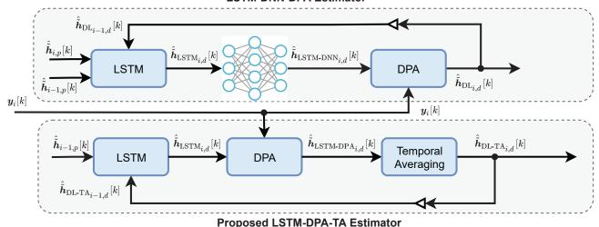
Fig. 1. LSTM-based IEEE 802.11p channel estimators block diagram.
