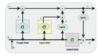
Fig. 2. LSTM unit architecture.
