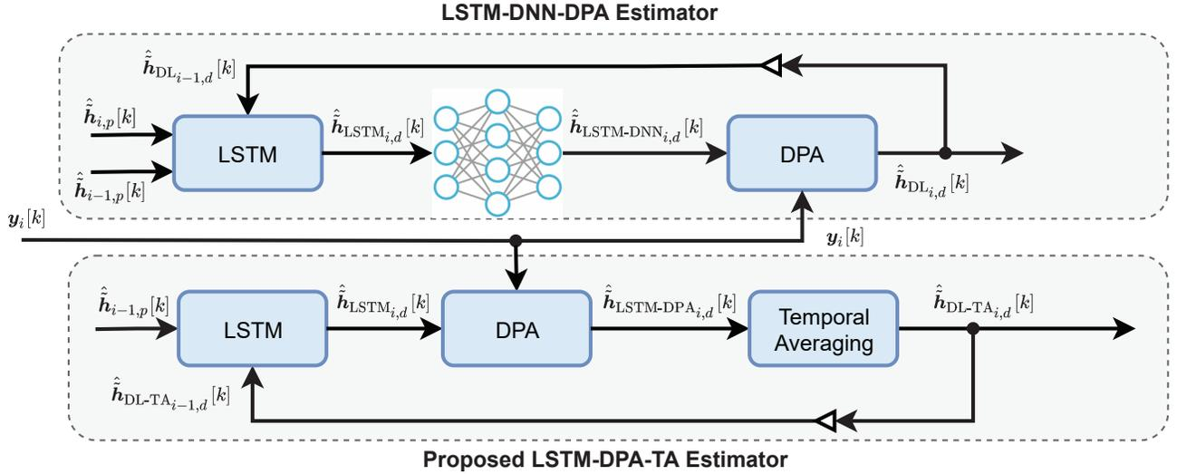
Fig. 1. LSTM-based IEEE 802.11p channel estimators block diagram.
