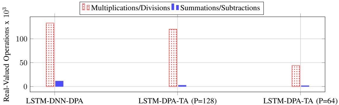
Fig. 4. Computational complexity of the studied channel estimators.
