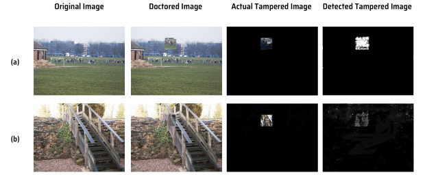
Fig. 3. Results of high quality ghost image inserted into low quality cover image (a) Grass field, (b) Stair.
