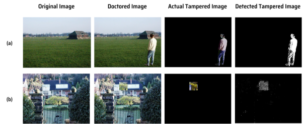
Fig. 4. Results of low quality ghost image inserted into high quality cover image (a) Man, (b) House.
