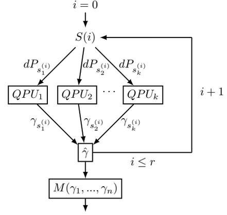
Fig. 2. A depiction executing a parallel program. The system starts at time  $i = 0$ , loading the programs specified by  $S(i)$  to the respective QPUs until all  $r$  rounds are ran. The outputs of the distributed programs are accumulated in an output vector  $\hat{\gamma}$  during execution. Finally  $M$  maps the collection of  $n$  outputs  $\hat{\gamma}$  to a single output.
