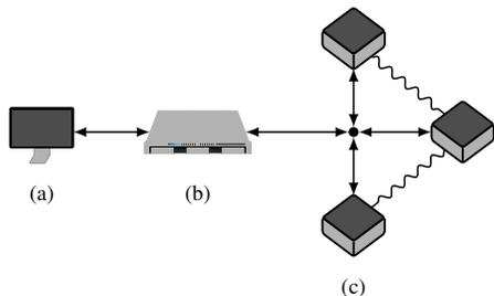
Fig. 3. The architecture used in Interlin-q: The client (a) constructs a circuit designed for a monolithic quantum computer and sends it to the controller (b). The controller remaps the circuit for the distributed system and constructs an execution schedule. Once complete, the respective control instructions are sent to each of the quantum computers in (c). The quantum computers execute the schedule and send the results back to the controller who processes the results to send back to the client.
