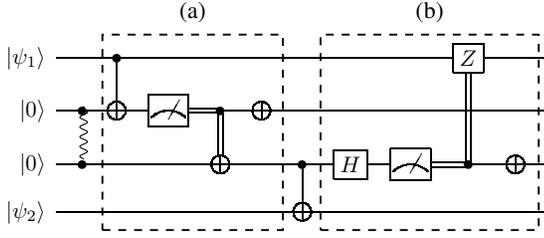
Fig. 1. Circuit diagram for a non-local CNOT gate between  $|\psi_1\rangle$  and  $|\psi_2\rangle$  where (a) is the cat-entangler sequence and (b) the cat-disentangler sequence.
