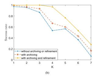
Fig. 5. RMSE( $\hat{\theta}$ ) (a) and success rate (b) results of three versions of MVESA versus model order K for M=15, T=10, and SNR= 10dB.
