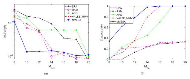
Fig. 9. RMSE( $\hat{\theta}$ ) (a) and success rate (b) results of all algorithms under varying  $M_{sel}$ s for K=3, T=10 and SNR= 10dB.
