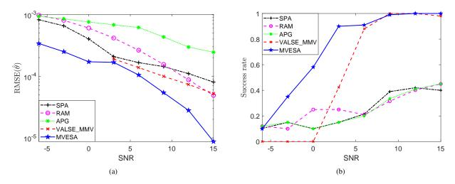
Fig. 6. RMSE( $\dot{\theta}$ ) (a) and success rate (b) results of all algorithms versus SNR for K=4,~M=15, and T=30.
