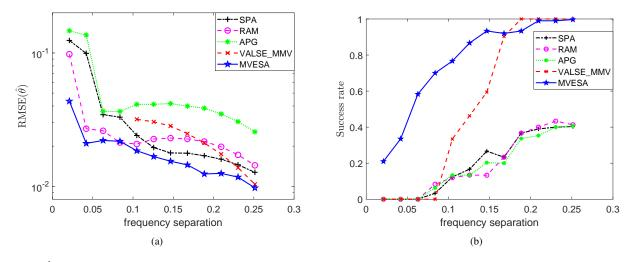
Fig. 8. RMSE( $\hat{\theta}$ ) (a) and success rate (b) results of all algorithms versus frequency separation for M=6, T=10, SNR= 10dB.
