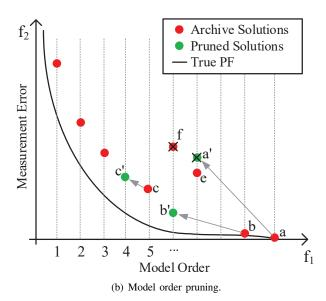
Fig. 3. Archiving and model order pruning mechanism. Vertical dotted lines refer to different model orders. Points labeled with cross symbols indicate being discarded.
