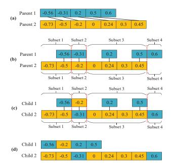
Fig. 2. Variable-length crossover. (a) Link the most similar counterparts between the two parents by black oblique lines. (b) Align the two parents, and segment the two parents into  $\bar{n}+1$  paired subsets by  $\bar{n}$  red dotted lines, where  $\bar{n}=3$  is the number of crossover points. (c) Crossover within each even paired subsets, respectively. (d) Glue subsets to produce two offsprings.
