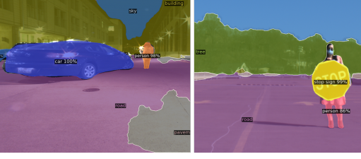
Figure 2: Image Segmentation: Metamoran uses image segmentation to identify the angular bounds along the azimuth and elevation axes for objects-of-interest – cars, persons, traffic signs – with semantic labels assigned.
