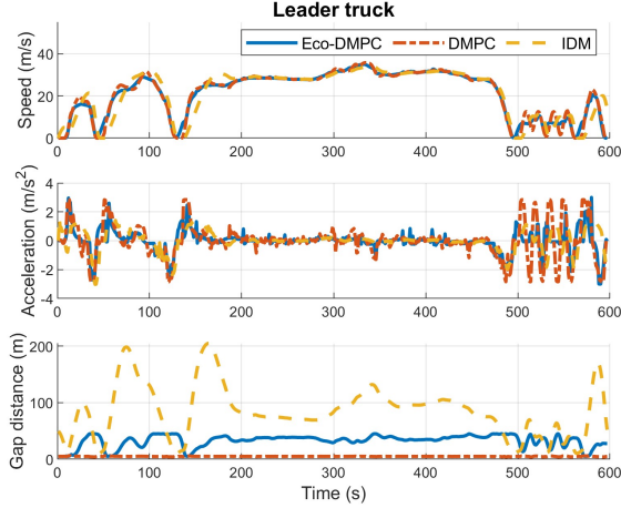
Fig. 3 The comparison of speed, acceleration, and gap distance profiles for the leader truck in Eco-DMPC, DMPC and IDM strategies.
