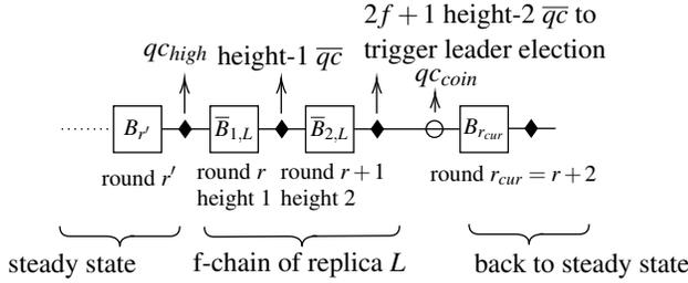
Figure 6: This figure illustrates one fallback-chain built by replica  $L$  in the asynchronous fallback of view  $v$ . The first fallback-block  $\bar{B}_{1,L}$  of height 1 contains the  $qc_{high}$ , and the second f-block contains the f-QC of the previous f-block.  $2f + 1$  height-2 f-QCs will trigger the leader election to form a coin-QC  $qc_{coin}$  that randomly selects a replica as the leader with probability  $1/n$ . Replicas continue the steady state from the f-chain by the leader.
