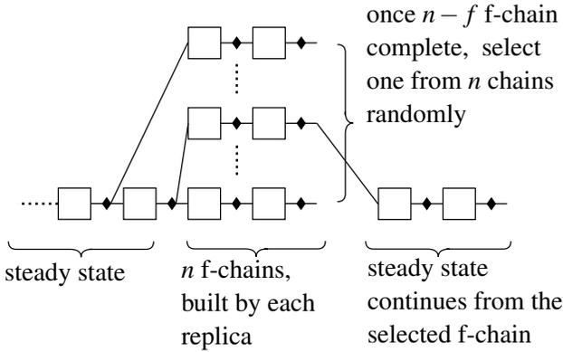
Figure 3: The high-level picture of the protocol. During the fallback, each replica acts as a leader and tries to build a certified fallback-chain (f-chain). When  $2f + 1$  f-chains are completed, one leader is randomly elected from  $n$  replicas, and all replicas continue the steady state chain from the f-chain built by the elected leader.
