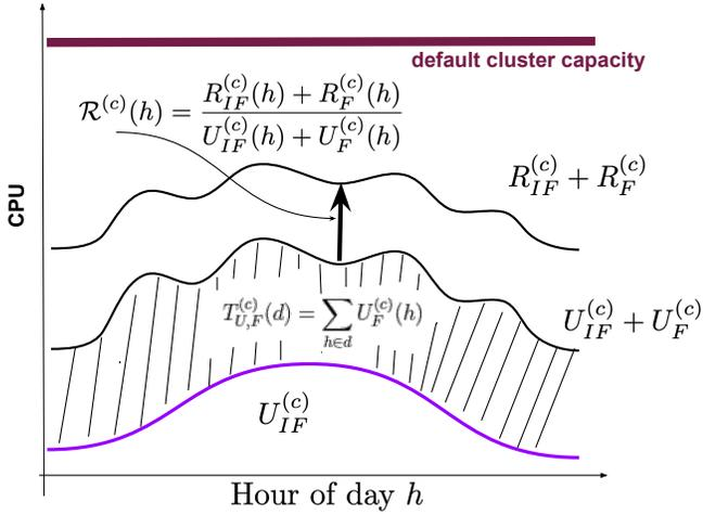
Fig. 6: Predicted load components for each cluster  $c$  fleetwide: inflexible usage daily profile  $U_{IF}^{(c)}(h)$ , daily flexible compute usage  $T_{U,F}^{(c)}(d)$ , all load reservation to usage ratio  $\mathcal{R}^{(c)}(h)$ .
