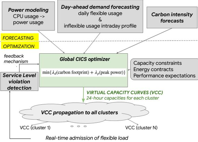
Fig. 4: Architecture of the Carbon-Intelligent Computing system.
