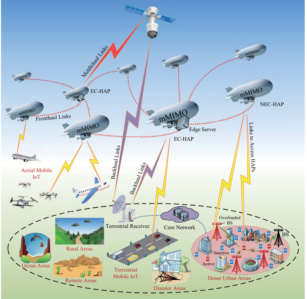
Fig. 1. The proposed edge computing paradigm for massive IoT connectivity, where the HAP-enabled aerial cell-free massive multiple-input multiple-output (mMIMO) network is employed and the potential application scenarios are illustrated.
