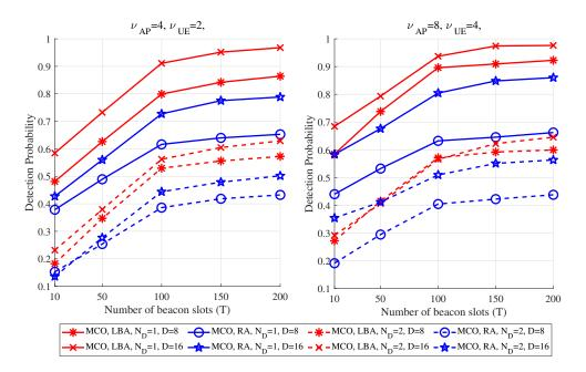
Fig. 3: Detection probability of the MCO BA proposed scheme versus the number of beacon slots T for different values of  $N_D$ ,  $\nu_{AP}$ ,  $\nu_{UE}$  and D. Parameters: M = 50, K = 15,  $N_{AP} = 32$ ,  $N_{UE} = 16$ ,  $n_{AP} = 8$ , and  $n_{UE} = 4$ .
