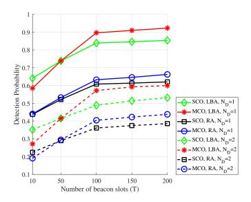
Fig. 2: Detection probability of the BA proposed schemes MCO and SCO versus the number of beacon slots T for two values of  $N_D$ . Parameters:  $M = 50, K = 15, N_{AP} = 32$ ,  $N_{UE} = 16, D = 8, n_{AP} = 8, n_{UE} = 4, \nu_{AP} = 8$ , and  $\nu_{UE} = 4$ .
