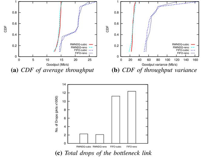
Figure 5: Elephant TCP flows performance: RWNDQ vs FIFO in a the Linux testbed with one bottleneck-link with new-reno and cubic TCP sources
