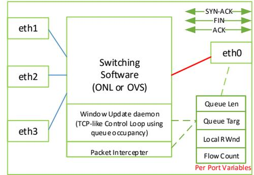
Figure 1: RWNDQ high level system-view design
