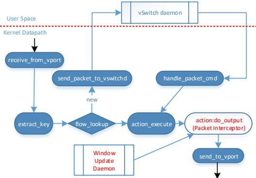
(b) OpenvSwitch-based RWNDQ packet processing pipeline
