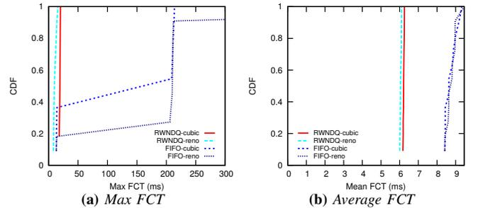
Figure 6: Mice TCP flows performance: RWNDQ vs FIFO in a the Linux testbed with one bottleneck-link with new-reno and cubic
