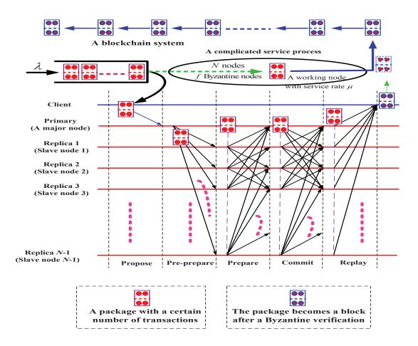
Figure 1: A useful relationship between the PBFT consensus and a queueing model
