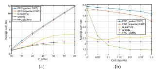
Fig. 3: (a) Average sum-rate vs. total transmission power at the BS  $(P_t)$  and (b) average sum-rate vs. minimum QoS requirement  $(Q_m)$ .
