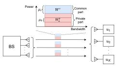
Fig. 1: An RSMA network consists of 1 M-antenna Base Station (BS) and K single-antenna users.
