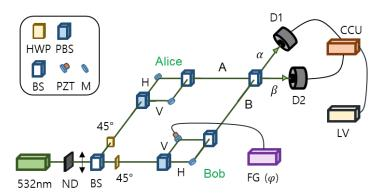
**Fig. 1**| **Schematic of Franson-type nonlocal correlation based on polarized coherent photons.** D: a single photon detector. CCU: coincidence counting unit. LV: Lab View software. H (V): horizontal (vertical) polarization. BS: beam splitter, M: mirror, PZT: Piezo-electric transducer, HWP: half-wave plate, PBS: polarizing BS.
