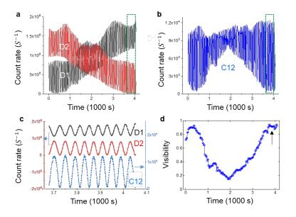
Fig. 2| Experimental results for Fig. 1. a Individual output counting rate for  $\alpha$  (D1) and  $\beta$  (D2). b Coincidence counting rate C12 for the output channels D1 and D2. c Expansion of (a) and (b) for the green dotted boxes: color matched. d Visibility between for  $\alpha$  (D1) and  $\beta$  (D2). The fast oscillation is due to the PZT-controlled phase  $\varphi$ , while the slow modulation is due to the global phase  $\theta$  between A and B in Fig. 1.
