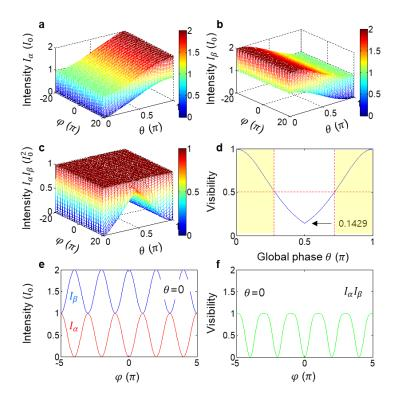
**Fig. 3** Numerical calculations for Fig. 2. a,b,c Output intensities  $I_{\alpha}$ ,  $I_{\beta}$ , and  $I_{\alpha}I_{\beta}$ . **d** Visibility between  $I_{\alpha}$  and  $I_{\beta}$ . The yellowish areas are for the quantum feature. **e** Details for (**a**) and (**b**). **f** Details for (**d**).
