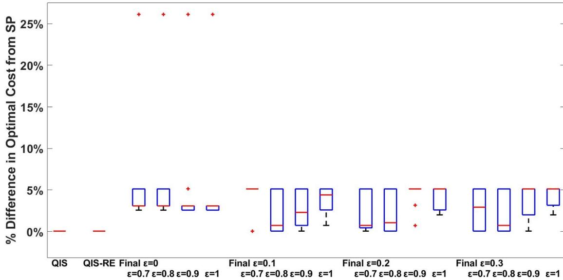
**Figure 3:** Comparison of % difference in optimal expected cost relative to the SP solution from simulating the optimal policies obtained in Epsilon Decay for different starting and final  $\epsilon$  values with reductions according to Equation 20 for 10 replications with QIS and QIS-RE. Boxes enclose the 50% interval, midlines indicate the median value, whiskers indicate the 90% interval, and outliers are shown as '+'.
