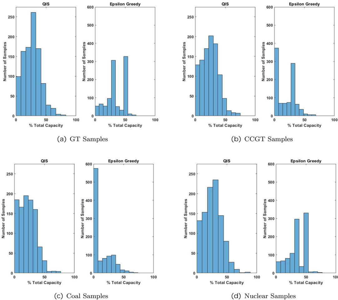
**Figure 4:** Final 1000 action samples for QIS and Epsilon Greedy as a percentage of Stage 1 new capacity for Natural Gas Combustion Turbine (4a), Combined Cycle Gas Turbine (4b), Coal (4c) and Nuclear (4d) technologies for one representative replication. Epsilon Decay and QIS-RE have not been shown because of similar behavior to Epsilon Greedy and QIS respectively. Note the change in the Y-axis scale between QIS and Epsilon Greedy.
