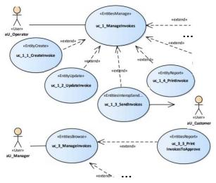
Fig. 9 Use case of invoice management system (partial from [19]).
