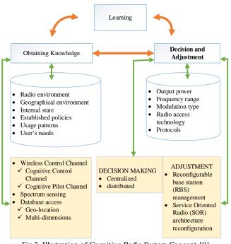
Fig.2. Illustration of Cognitive Radio System Concept [9]
