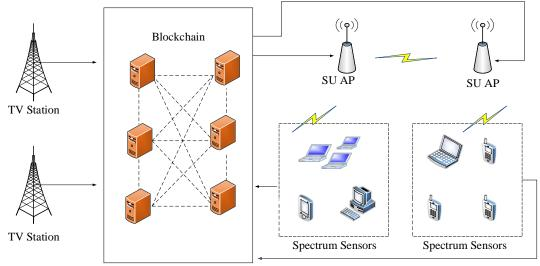
Fig. 4 DLT Actors and Components for use Case of Spectrum Sharing in TVWS
