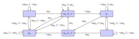
Fig. 1: Synthesized LTS for the satellite specification.
