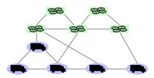
Figure 6: Network of non-homogeneous agents operating on multiple time scales. Faster aerial vehicles are shown in green squares, and slower ground vehicles are shown in blue ellipses.
