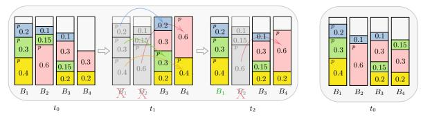
(a) A valid solution: four items are packed at time  $t_0$ . Bins  $B_1$  and  $B_2$  fail at time  $t_1$ , and standby replicas in other bins replace primary replicas in the failed bins.  $B_1$  recovers at  $t_2$ , and the algorithm gives back the primary status to replicas in  $B_1$ .
