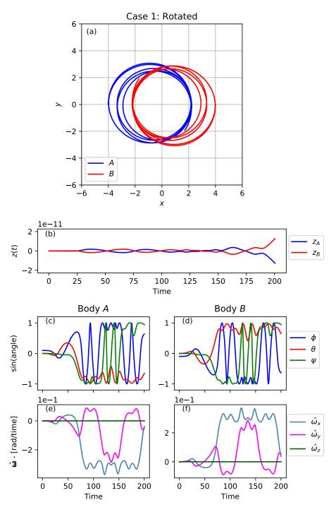
Fig. 2 For case 1, where the spheroids are initially rotated about their respective x-axes. (a) The orbits of spheroids A and B in the inertial frame projected into the xy-plane. (b) The z-position of the spheroids as a function of time. (c,d) The rotation angles of bodies A and B as sine functions. (e,f) The angular velocity in the body-fixed frames of bodies A and B as a function of time. The unit of the angular velocity  $\hat{\boldsymbol{\omega}}$  is radians per unit time.
