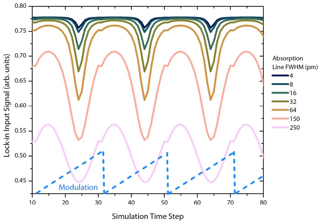
Figure 4: Simulated lock-in amplifier input signal ( $V_{in}$ ) over time for various CO<sub>2</sub> absorption line FWHM values. The modulation signal is shown as a blue dashed line. The additional periodic features at time steps 31, 51, and 71 are artifacts of the sawtooth modulation.
