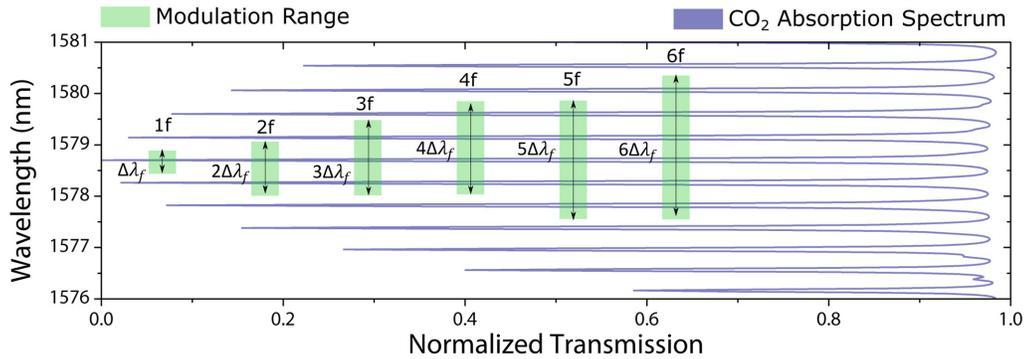
Figure 11: (a) Absorption spectrum of CO<sub>2</sub> overlaid with FFP filter modulation ranges for higher order harmonic radial velocity sensing. The height of the green bars represent multiples of the fundamental modulation range, with the harmonic frequency marked above each bar.
