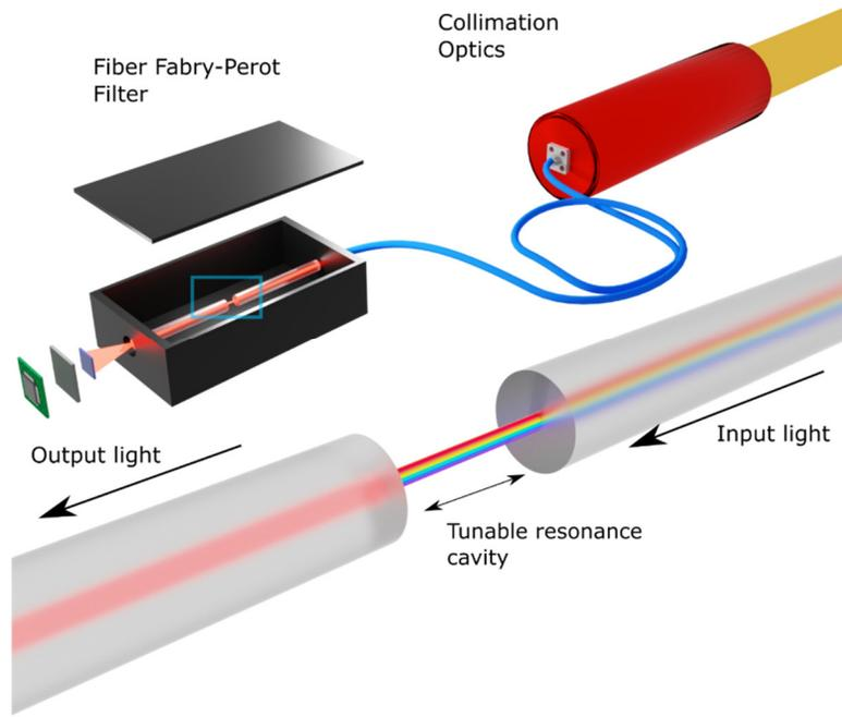
Figure 1. Illustration of the operation of a FFP filter in a free-space coupled system.
