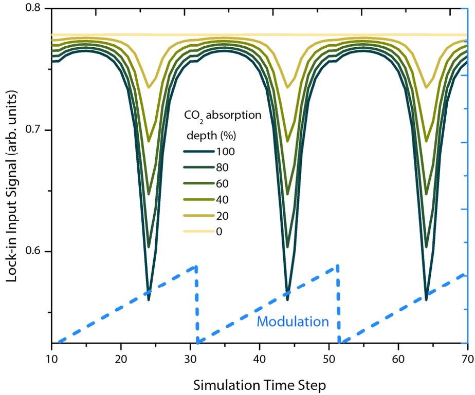
Figure 3: Simulated lock-in amplifier input signal ( $V_m$ ) over time for various CO<sub>2</sub> absorption depths. The sawtooth modulation function is shown as a dashed blue line.
