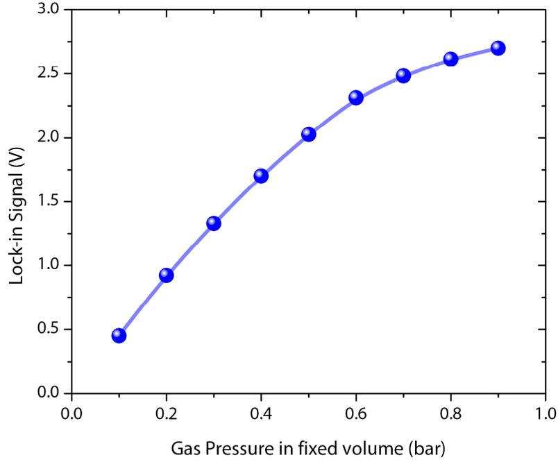
Figure 8: Experimental  $V_{out}$  signal as a function of gas pressure in the Herriott cell. Pressure and lock-in signal uncertainties for the pressure and lock-in voltage are 10 mbar and 0.01 V, respectively, and are too small to be shown here. The curve is used as a guide to the eye.
