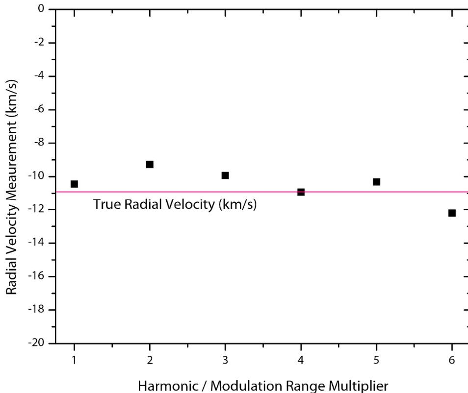
Figure 13. Radial velocity extracted from the Venus spectrum for increasing lock-in demodulator harmonics  $n_n$ . The true radial velocity of Venus at the time of acquisition is shown as the colored line.
