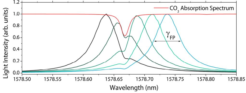
Figure 2. Simulated transmission spectrum of the tunable Fabry-Pérot filter as it is tuned across the single CO<sub>2</sub> spectral line at 1578.66 nm (red).
