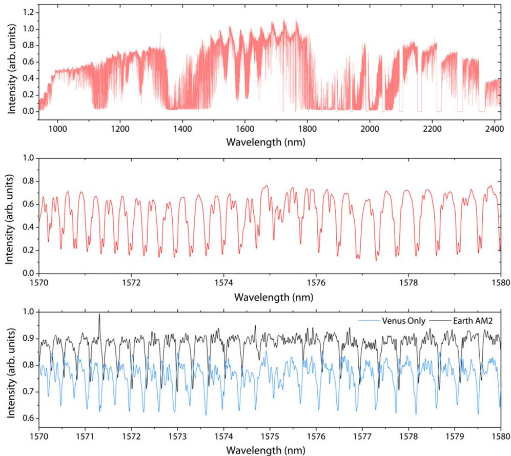
Figure 10: (a) Near-infrared spectrum of Venus taken at an air mass of  $\sim 2$  through Earth's atmosphere. (b) Measured high-resolution spectrum including contribution from both Earth and Venus. (c) Processed spectrum of Venus (blue) after correcting for the telluric lines using a measured AM2 spectrum.
