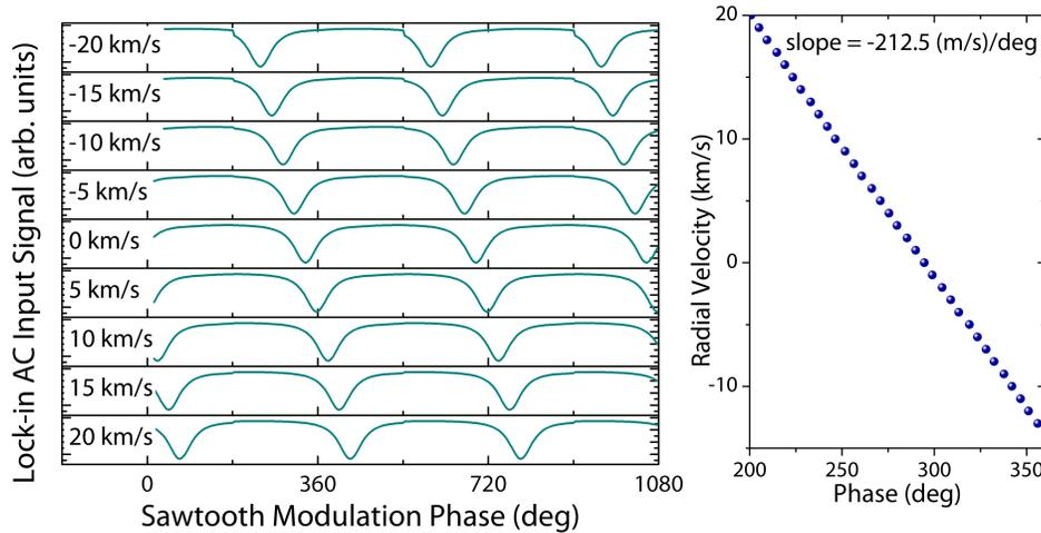
Figure 9: (a) Total light output from the FFP filter (AC input to the lock-in amplifier) as a function of the phase of the sawtooth modulation of the central transmission wavelength for a range of radial velocities. The artifact halfway through the modulation arises from the discontinuity of the sawtooth function. (b) The phase of the signal as a function of radial velocity. The slope can be used to determine the radial velocity of the target using the measured phase of the AC signal.
