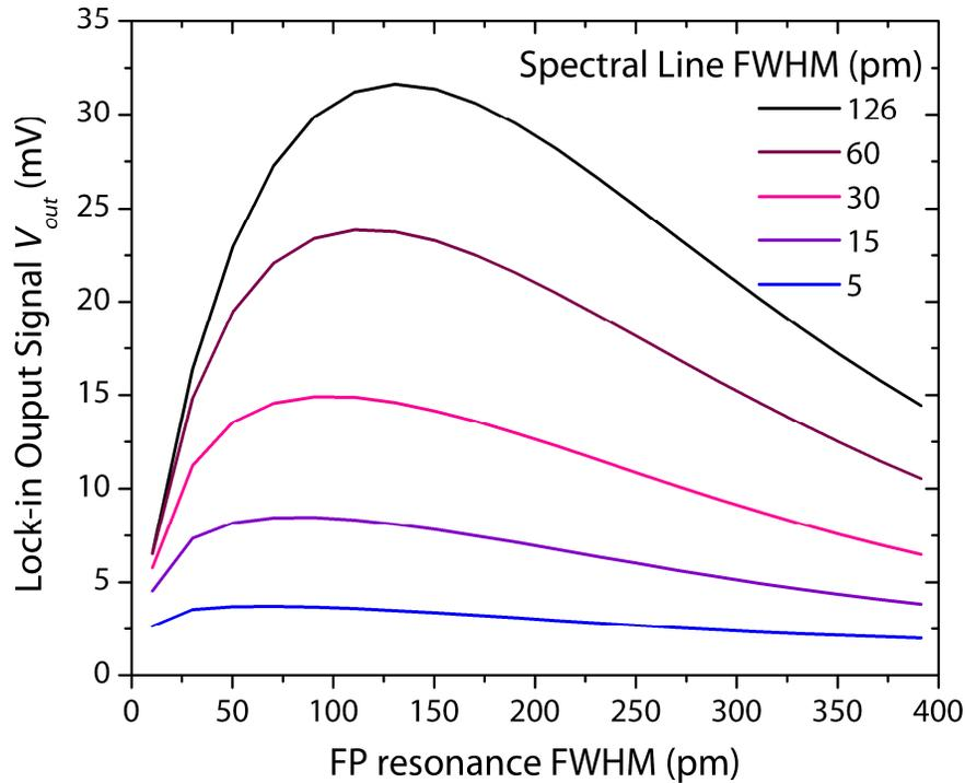
Figure 5: Simulated lock-in amplifier output ( $V_{out}$ ) signal as a function of the absorption line FWHM. The voltage of the lock-in amplifier is arbitrary in scale as it depends on the signal gain.
