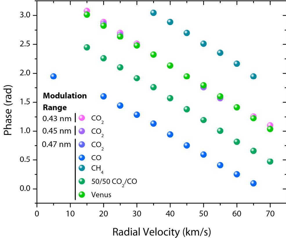
Figure 12: Phase shift as a function of radial velocity of various redshifted spectra using the 6<sup>th</sup> order lock-in amplifier harmonic over a modulation range of  $6 \times \Delta\lambda_f$  and a harmonic order of 6 times the average spacing between adjacent CO<sub>2</sub> lines (2.83 nm) centered at 1580.2 nm. The value of  $\Delta\lambda_f$  is varied from 0.43 nm to 0.47 nm for the CO<sub>2</sub> spectrum.
