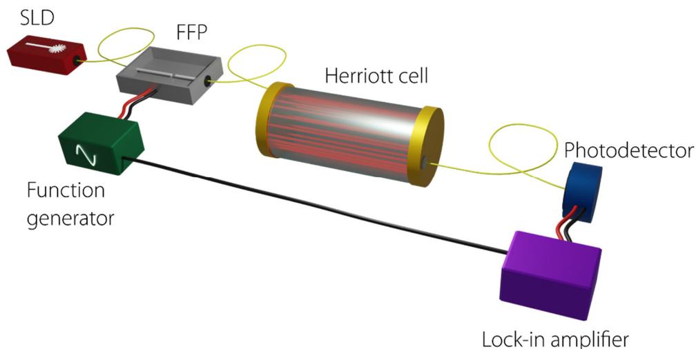
Figure 7: Schematic illustration of the optical and electrical experimental benchtop system. The grey box indicates the fiber Fabry-Pérot filter. The yellow wires represent polarization maintaining optical fibres.
