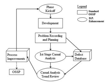
Fig. 1. Defect prevention strategy for software development process; Here in the Figure, OSSO stands for organization standard software process
