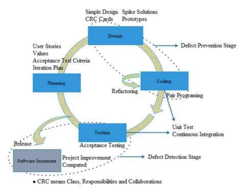
Fig. 2. Defect detection and prevention model in Extreme programming
