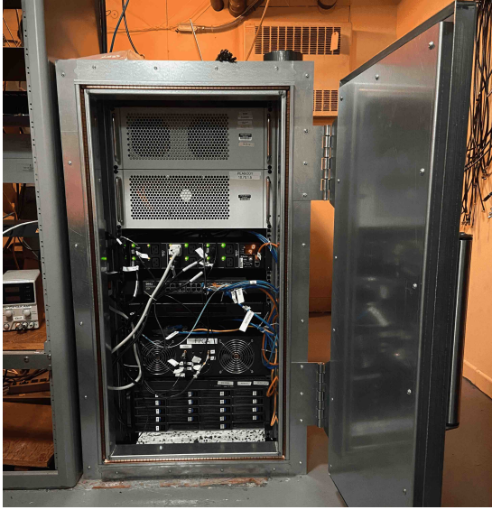
Figure 5. RF-shielded rack located in the main control room at ARO. The rack includes (from top to bottom): controller node, analysis node, PDU, main switch, GPS unit, ICE/FPGAs, and recording node.
