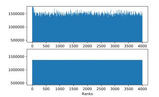
Figure 2: Visualizing the load distribution for the Fock matrix computation for the Ubiquitin protein. Results from: Top, current assignment on NWChemEx. Bottom, submodular assignment.
