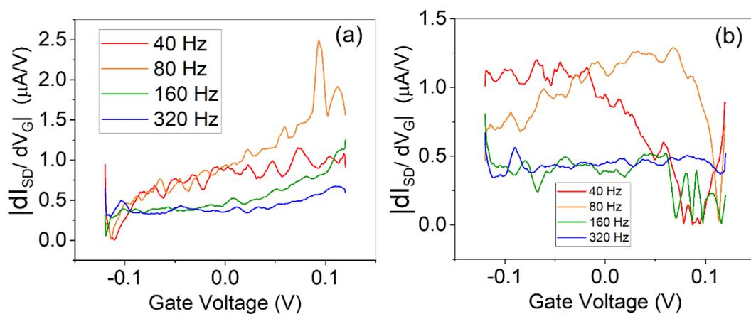
Figure S3: Variation in the derivative of source-drain current with the applied gate voltage during the (a) increasing and (b) decreasing values of the gate voltage.
