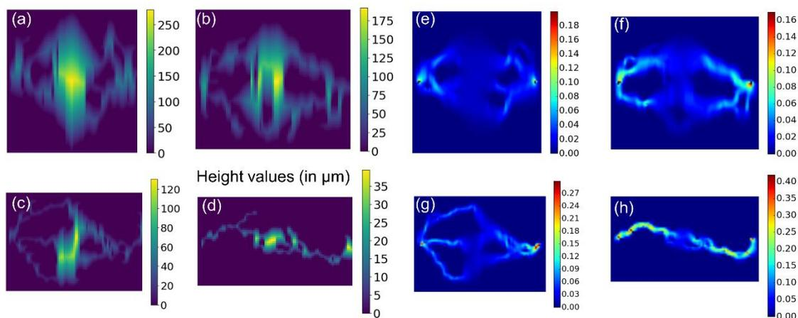
Figure S2: (a-d) 3-d morphology of dendrites based on multiple cylinder assumption and corresponding (e-h) normalized current density map for the dendrite obtained at  $f_p = 40\text{-}320$  Hz based on image analysis and electrical simulations.
