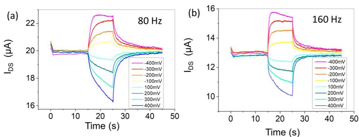
Figure S4: Source-Drain current responses for dendritic OECTs grown at (a)  $f_p = 80\text{Hz}$  and (d)  $f_p = 160\text{ Hz}$  with pulse amplitude from  $-0.4$  to  $0.4\text{ V}$ .
