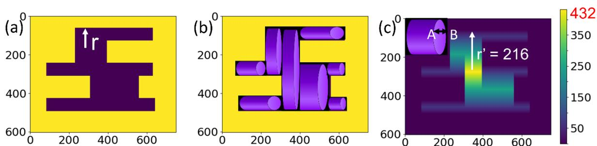
Figure S1: (a) An example of a 2d image, (b) reconstructed 3d image based on cylindrical shapes, (c) 3d profile of the image.
