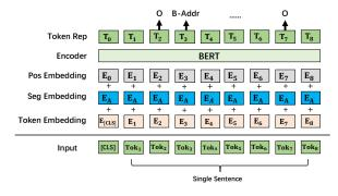
Figure 3: The sequence labeling BERT model for NER.
