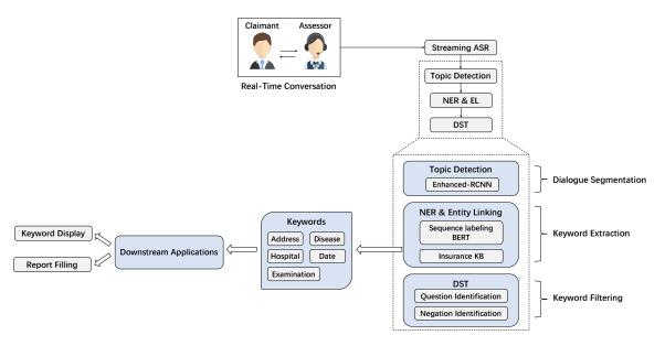
Figure 2: The Architecture of Intelligent Insurance Assessment System.
