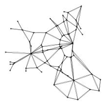
Fig. 3: EMA transportation network composed of 74 nodes , 258 arcs, 581 lanes, and 1113 OD pairs.
