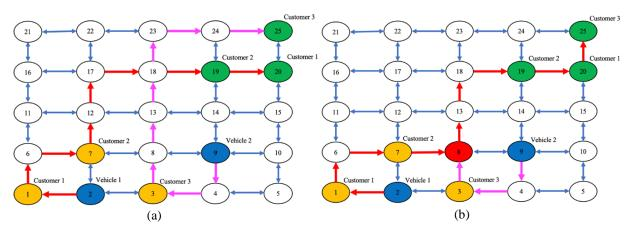
Figure 3. Optimal routes under (a) no transfers with 2 vehicles, and (b) transfers allowed with 2 vehicles.
