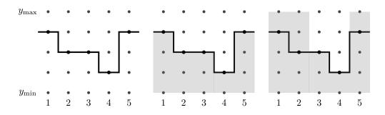
**Figure 1:** The no-good (left), monotonic (centre), and local cuts (right). The lattice points correspond to the binary variables. The solutions that the bound is valid at correspond to taxi-cab-like paths through the shaded region.
