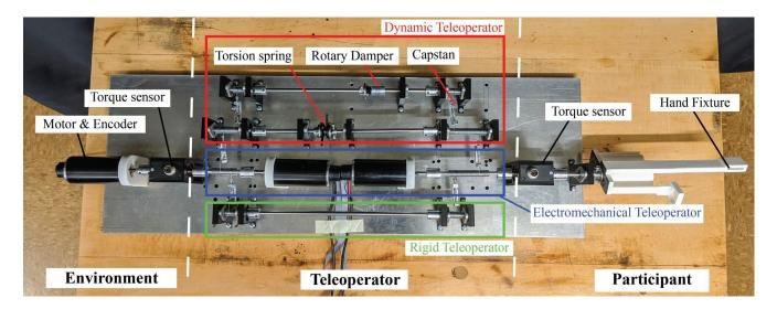
Fig. 1. Experimental setup with the three modules: 1) Participant- custom 3D printed hand fixture and torque sensor, 2) Teleoprator including three transmissions - rigid mechanical (green), electromechanical (blue), and dynamic mechanical (red), and 3) Environment - DC motor and encoder for virtual environment rendering and torque sensor.
