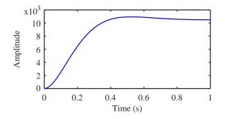
Fig. 4. Step response illustrating the inherent damping the participant feels while using the rigid mechanical teleoperator transmission to explore free space
