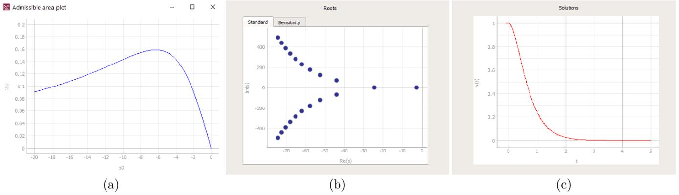
Fig. 2. Example of the usage of  $P3\delta$  in the “Control-oriented MID” mode for the delay-differential equation (3) with  $\omega = 2\pi$ . (a) Admissible region. (b) Roots of the characteristic quasipolynomial. (b) Numerical simulation of a solution with initial condition  $x(t) = 1$  for  $t \leq 0$ .
