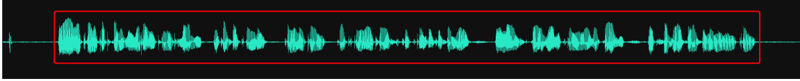
Figure 1: An example of how our rule-based voice activity detection model works on the waveform. Note that only the part in the red box will be retained as a valid fragment.
