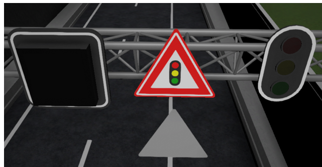
Figure 6.18: From left to right: a matrix sign, a J32-sign with its cover plate that simulates it turning off and a traffic light.
