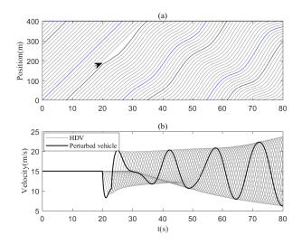
Fig. 3. (a) Trajectory of all vehicles (the trajectory of the perturbed vehicle and vehicle no. 20 are, respectively, shown by black and blue lines) when there is no CAV in the platoon (a disturbance is added to the acceleration of vehicle 7 at t = 20 s); (b) Velocity profile of vehicles.
