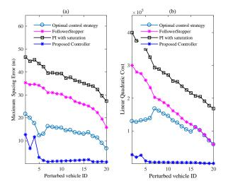
Fig. 5. Comparison of the results for four different control strategies; (a)  $\max_t |s_1(t) - s_1^*|$  w.r.t. the index of the perturbed HDV; (b) Energy of the performance output, i.e.,  $||z(t)||_2 = \int_{t=0}^{\infty} x^T(t) \mathcal{T}x(t) + u^T(t)\mathcal{Q}u(t)$ , w.r.t. the index of the perturbed HDV.
