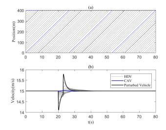
Fig. 4. (a) Trajectory of all vehicles (the trajectory of the perturbed vehicle and vehicle no. 20 are, respectively, shown by black and blue lines) when there is one CAV under the proposed control is Section IV-C (a disturbance is added to the acceleration of vehicle 7 at t = 20 s); (b) Velocity profile of vehicles.
