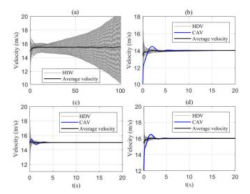
Fig. 2. (a) Velocity profile of vehicles when they are all HDVs; (b)–(d) Velocity profile of vehicles when the 1<sup>st</sup> vehicle is a CAV under the proposed control in Section IV-C, and  $v^*$  is 15, 16, and 14 for (b), (c), and (d), respectively.
