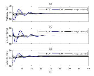
Fig. 6. (a)–(c) Velocity profile of vehicles when there is one CAV under the proposed control in Section V in the presence of disturbances and the parametric uncertainties, and  $v^*$  is 14, 15, and 16 m/s for (a), (b), and (c), respectively.
