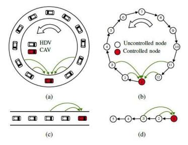
Fig. 1. (a)–(b) Schematic of a mixed traffic system on a ring-road and the corresponding graph; (c)–(d) Schematic of a mixed traffic system on an open-road and the corresponding graph.
