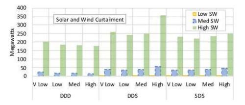
Figure 4: Average curtailed solar and wind energy.
