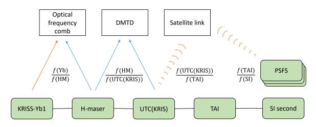
**Figure 1.** Frequency chain schematic diagram for the absolute frequency measurement relative to the SI second (Terrestrial time, TT). DMTD: multi-channel dual-mixer time difference, PSFS: primary or secondary frequency standards
