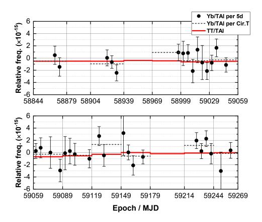
**Figure 8.** The relative frequency offset from the 2017 CIPM-recommended frequency of the 5-day-grid KRISS-Yb1 measurement values relative to TAI (black dots), the monthly determined KRISS-Yb1 frequency (black dashed lines), and the duration of the TAI scale interval *d* (TT relative to TAI) reported in Circular T (thick red lines).
