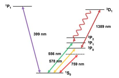
Figure 3. Optical transitions between energy levels used in the Yb optical clock.
