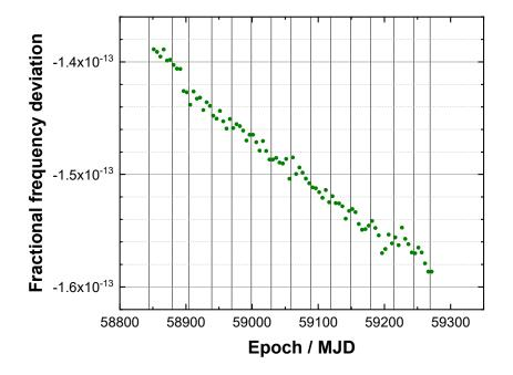
**Figure 6.** Fractional frequency deviation of the HM (H5626) measured by TT during the absolute frequency measurement campaign (MJD 58844 ~ 59269) with the average drift value of  $-4.5 \times 10^{-17}$ /d. The vertical solid lines represent the separated interval for each Circular T. The drift rate and its uncertainty for each month-grid of the Circular T was determined by a linear fit for 3 months (including the previous and the next month).
