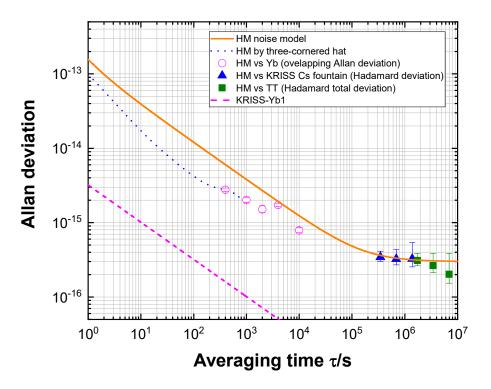
**Figure 7.** Frequency instability of the HM (H5626) measured by three-cornered hat method using two other HMs (blue dotted line), by the Yb optical lattice clock (pink open circles), by the KRISS Cs fountain clock (blue triangles), by TT (green squares). The pink dashed line represents the stability of the Yb optical lattice clock.
