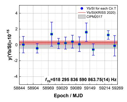
**Figure 9.** The relative frequency offset of the monthly determined KRISS-Yb1 absolute frequencies for each Circular T (blue dots) from the 2017 CIPM-recommended frequency. Blue error bars represent the total uncertainties of each month and light green error bars represent
