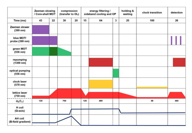
**Figure 4.** Experimental sequence of KRISS-Yb1. OL: optical lattice, OP: optical pumping for the spin-polarization of the initial state of trapped Yb atoms, H coil: Helmholtz coil, AH coil: anti-Helmholtz coil, Q-axis: quantization axis. In the dark green region, the frequency of the 556 nm laser was modulated for better transfer of atoms to the green MOT.
