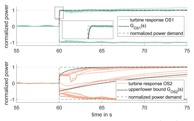
Figure 8: Normalized step response for demand steps of  $\Delta P_{ref}$  at constant wind speeds of  $v = \{8, 12, 16\}$  m/s
