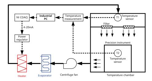
Figure 3: Schematic of the air temperature control system.
