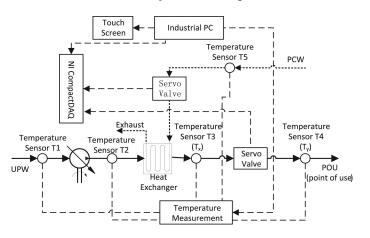
Figure 5: Schematic of the immersion liquid temperature control system [27].
