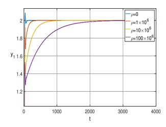
Figure 6: Step response of PI/P cascade control.
