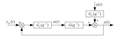
Figure 1: A single closed-loop control system.
