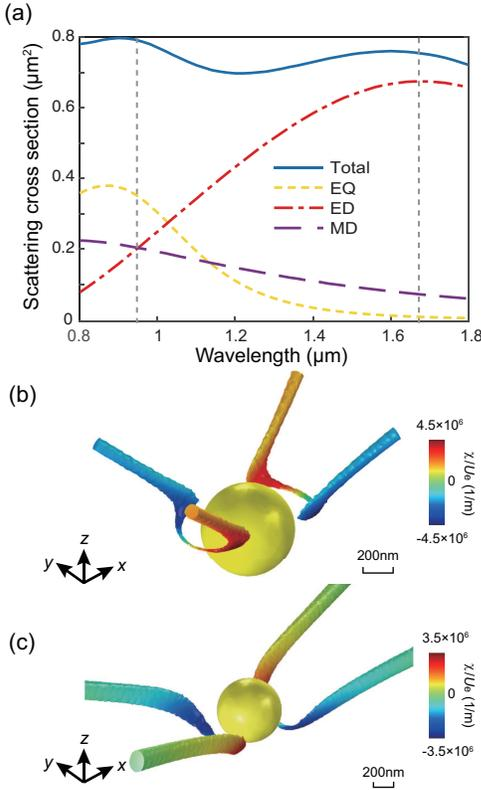
FIG. 1. (a) Scattering cross section of the gold sphere illuminated by a  $x$ -polarized plane wave propagating in  $z$  direction. (b) Type-I C line of the gold sphere at  $\lambda = 950$  nm. (c) Type-II C line of the gold sphere at  $\lambda = 1680$  nm. The color of the C lines denotes the normalized optical chirality  $\chi/U_e$ .
