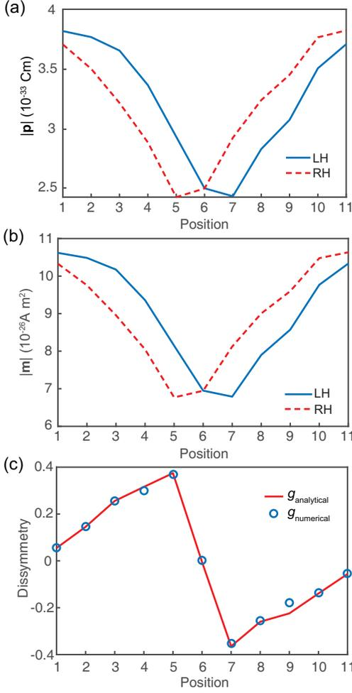
FIG. 6. Amplitude of (a) the electric dipole moment  $\mathbf{p}$  and (b) the magnetic dipole moment  $\mathbf{m}$  as a function of the position for the Type-II C line. (c) Comparison between the analytical and numerical results of the dissymmetry factor.
