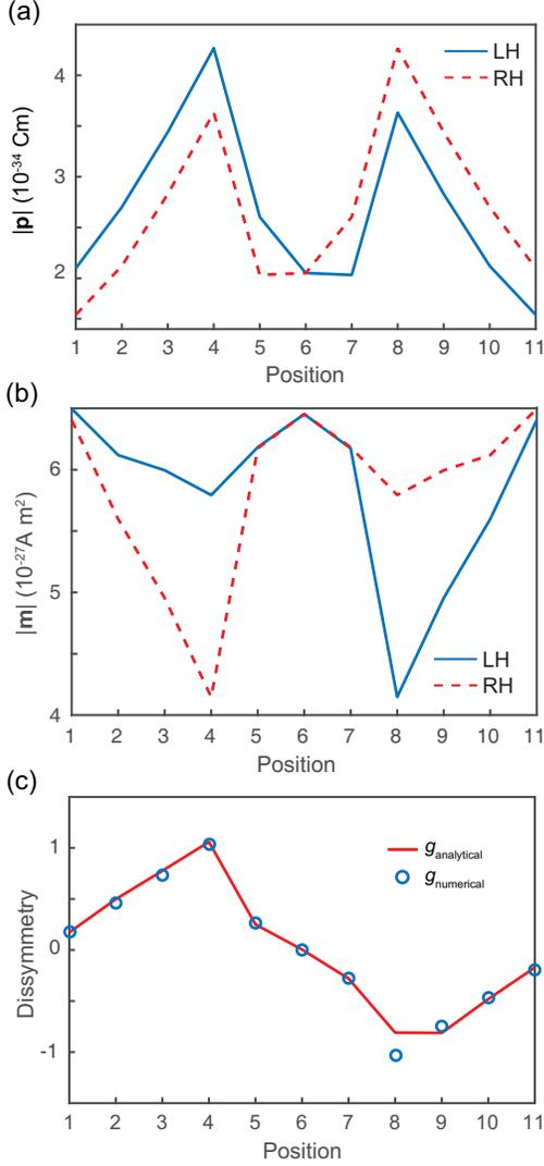
FIG. 3. Amplitude of (a) the electric dipole moment  $\mathbf{p}$  and (b) the magnetic dipole moment  $\mathbf{m}$  as a function of the position for the Type-I C line. (c) Comparison between the analytical and numerical results of the dissymmetry factor.
