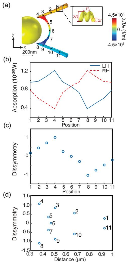
FIG. 2. (a) Schematic for chiral discrimination by the Type-I C line. A two-pitch gold helix serves as the chiral particle and is located at the positions labeled as 1-11. Its inner radius  $r = 5$  nm, outer radius  $R = 10$  nm, pitch  $p = 15$  nm. (b) The absorption of the LH and RH helices as a function of the position. (c) The dissymmetry factor as a function of the helix's position. (d) The dissymmetry factor as a function of distance from the gold nanoparticle.
