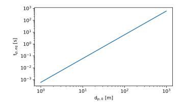
**Figure 9.** The time required to reach the equilibrium diameter,  $d(t_{p,eq}) = d_{p,eq} = 0.5 d_{p,0}$ , as a function of initial particle diameter  $d_{p,0}$ .
