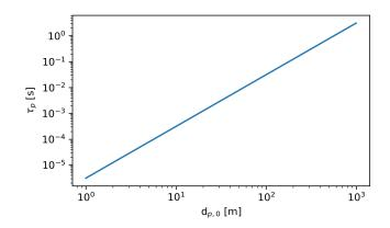
**Figure 8.** The stopping time  $\tau_p$  as a function of initial particle diameter  $d_{p,0}$ . The particle density is constant at  $\rho_p = 1000 \text{ kg/m}^3$ . The fluid dynamic viscosity  $\mu_f$  is computed using Sutherland's Law (see Eq. 1) at the initial bus temperature  $T_{f,0} = 288.15 \text{ K}$ .
