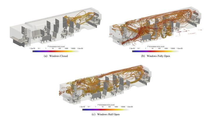
**Figure 19.** Volumetric rendering of regions of non-zero VMET comparing the dispersion of particles when passenger 14 sneezes for the a) windows closed case, b) windows fully open case, and c) windows half open case.
