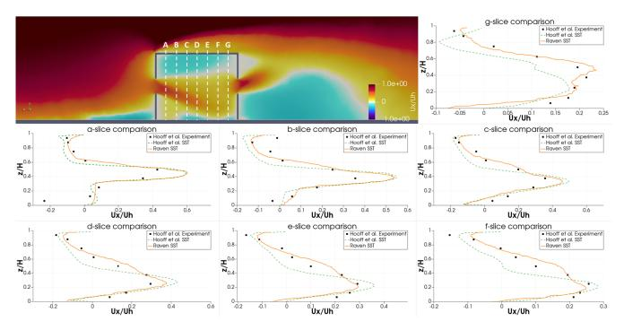
**Figure 13.** Vertical velocity profiles extracted from RavenCFD simulation results at varying position inside the room embedded in cross-flow, compared with the results of Ref. 20.
