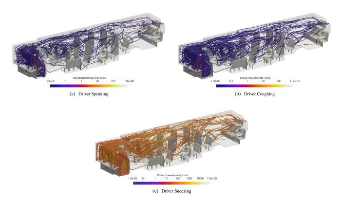
**Figure 16.** Volumetric rendering of regions of non-zero VMET for the fiducial case, comparing three injection events of the bus driver a) speaking, b) coughing, and c) sneezing.
