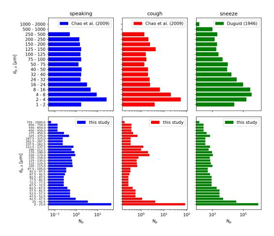
**Figure 11.** Particle number distributions of initial particle diameter  $d_{p,0}$ . The data from Refs. 14 and 15 is resampled to a finer particle size distribution for this study. Note that the number of particles reported is a sum over each sampled diameter range.
