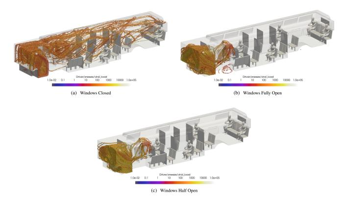
**Figure 18.** Volumetric rendering of regions of non-zero VMET comparing the dispersion of particles when the bus driver sneezes for the a) windows closed case, b) windows fully open case, and c) windows half open case.
