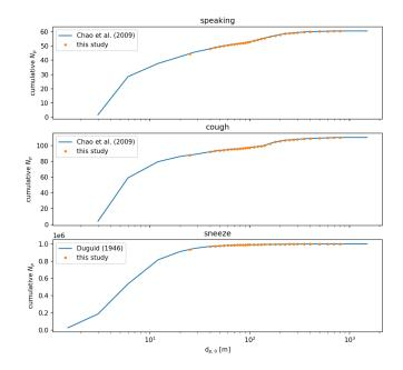
**Figure 10.** Comparison of cumulative particle number distributions between the source data in Refs. 14 and 15 and the resampled size distributions for this study.
