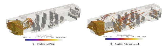
**Figure 21.** Volumetric rendering of regions of non-zero VMET comparing the dispersion of particles when the bus driver sneezes for the a) windows half open and b) windows alternate open B.
