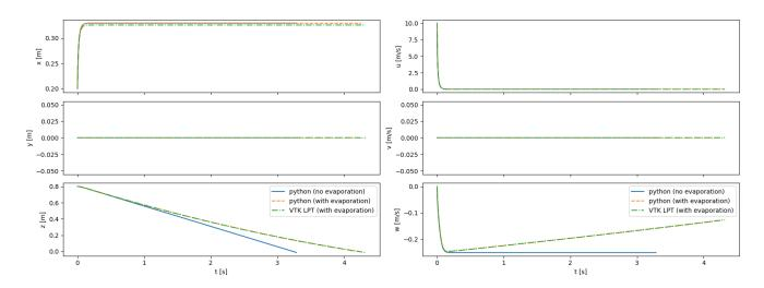
**Figure 14.** Comparison between trajectories computed with Python, both with and without the evaporation model; and with the VTK LPT algorithm. Results are shown for a 100  $\mu$ m particle injected into a static room with initial velocity of 10 m/s in the +x direction. The particles are integrated until they impact the ground.
