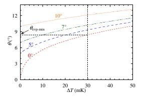
Figure 15: Value of  $\theta$  as a function of  $\Delta T$  for different  $\theta_{\text{micro}}$  computed for pentane at 1 bar. The curve for  $\theta_{\text{micro}} = 0$  corresponds to  $\theta_{\text{evp-min}}(\Delta T)$ .
