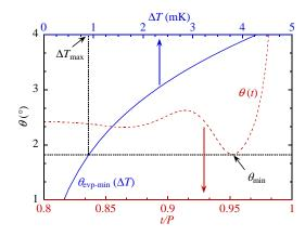
Figure 12: Apparent contact angle  $\theta$  calculated for  $\theta_{micro} = 0$  as a function of superheating  $\Delta T$  (example of pentane at 1bar, same as in Fig. 15) plotted together with the apparent contact angle variation during meniscus oscillation. The latter is a curve for initial value  $10^{\circ}$ , the same as at the inset of Fig. 4a.
