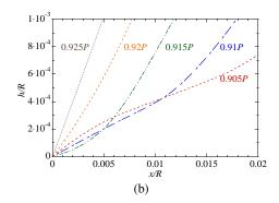
Figure 4: Contact angle variation for  $Ca_0 = 10^{-3}$ ,  $\tilde{P} = 50$ . (a) Variation of contact angle during an oscillation for different values of  $\theta_i$ . The inset shows enlarged undulating portions of the curves. (b) The interface shape variation near the contact line around t = 0.913P where  $\theta_{\min}$  is attained for  $\theta_i = 20^\circ$  (cf. the inset to Fig. 4a).
