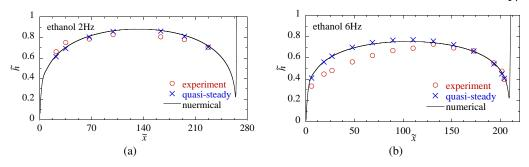
Figure 10: Liquid film thickness: comparison of the experimental data of Youn *et al.* (2018), quasi-steady estimation with Eq. (3.12) and numerical results for ethanol.
