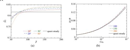
Figure 7: Average thickness of the liquid film at t = 0.5P;  $\langle h_q \rangle$  is shown for comparison. (A) Value of  $\langle \tilde{h} \rangle$  as a function of oscillation period for different  $\theta_i$  and for  $Ca_0 = 10^{-3}$  and (b) value of  $\langle h \rangle$  as a function of  $Ca_0$  for different  $\tilde{P}$  and for  $\theta_i = 20^{\circ}$ .
