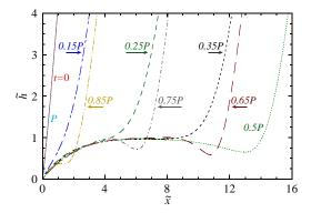
Figure 2: Periodic interface shape variation at oscillation for  $\tilde{P} = 50$ ,  $Ca_0 = 10^{-3}$  and  $\theta_1 = 20^{\circ}$ . The labels give the times corresponding to each profile, and arrows indicate the meniscus motion direction.
