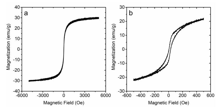
Figure S1. Static magnetic hysteresis loops of air-dried IPG30 MNPs measured by a PPMS. The field range is (a) -5000 – 5000 Oe and (b) -500 – 500 Oe, respectively.
