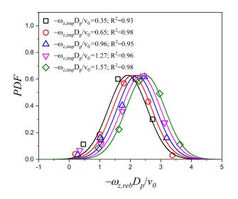
Figure 21: Probability density of the spanwise nondimensional rebound angular velocity. The symbols are the simulation results, and the lines are curve fitting results by equation (17), where  $R^2$  is used to evaluate the fitting results.
