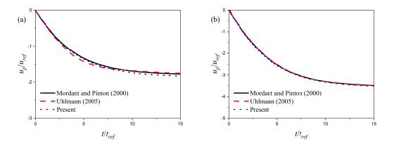
Figure 2: Comparison of the settling velocity for different density ratios: (a)  $\rho_p/\rho_f = 2.56$  and (b)  $\rho_p/\rho_f = 7.71$ . The settling velocity and the time are normalized by  $u_{ref} = \sqrt{D_p |g|}$  and  $t_{ref} = \sqrt{D_p / |g|}$ , respectively.
