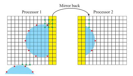
Figure 6: Two-dimensional illustration of data transmission in particle-fluid interaction calculations. The blue circle is the finite-sized particle. The yellow region is the ghost-cell region. The red points are the Lagrangian points on the particle surface. The green points are the Eulerian grid points affected by a Lagrangian point.
