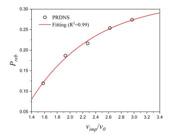
Figure 18: Rebound probability of the impact particles. The symbols are the simulation results, and the line is curve fitting result by equation (14).  $R^2$  is the coefficient of determination, which is used to evaluate the fitting results.
