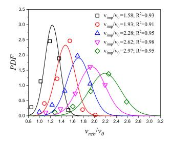
Figure 19: Probability density of the nondimensional rebound velocity. The symbols are the simulation results, and the lines are curve fitting results by equation (15).  $R^2$  is the coefficient of determination, which is used to evaluate the fitting results.
