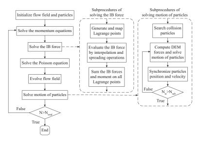
Figure 7: The flowchart of the hybrid parallel approach in PRDNS with the direct-forcing immersed boundary method.
