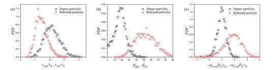
Figure 17: Probability density of the nondimensional quantities of the impact and rebound particles: (a) impact and rebound velocity, (b) impact and rebound angle and (c) impact and rebound spanwise angular velocity.
