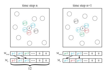
Figure 8: Sketch of the memory optimization method with the dense packing concept.  $M_p$  and  $M_{temp}$  are two arrays to store the collision information at time steps n and n-1, respectively. The circles in different colors indicate particles in different collision events.
