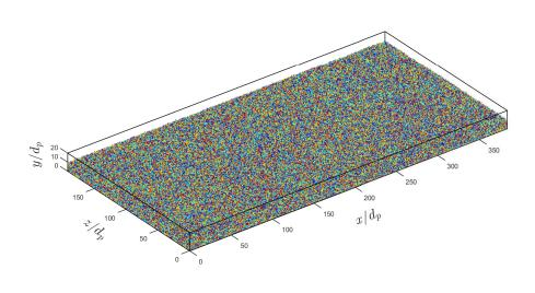
Figure 9: The sketch of sediment transport case with over a million sphere particles.
