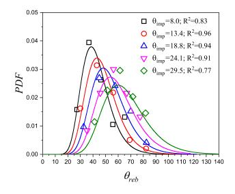
Figure 20: Probability density of the rebound angle. The symbols are the simulation results, and the lines are curve fitting results by equation (16), where  $R^2$  is used to evaluate the fitting results.
