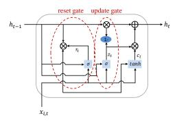
Fig. 5. The structure of a GRU cell.
