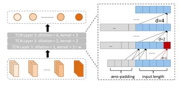
Fig. 4. The architecture of TCN for processing the historical weekly period.
