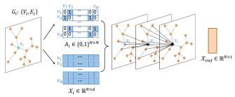
Fig. 3. The subgraph based on central road segment  $v_i$  is  $G_i$ . With a two-layer GCN, the output for each sub-graph at a specific time is a vector with dimension N.
