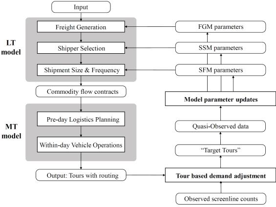
Fig. 6 The overview of screenline-based two-step calibration for SimMobility Freight.
