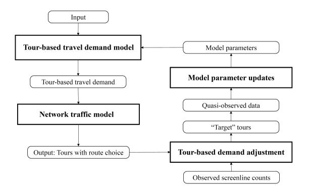
Fig. 1 The overview of Screenline-based Two Step Calibration. The left side is the flow of a simulation model and the right side is the flow of proposed calibration method.
