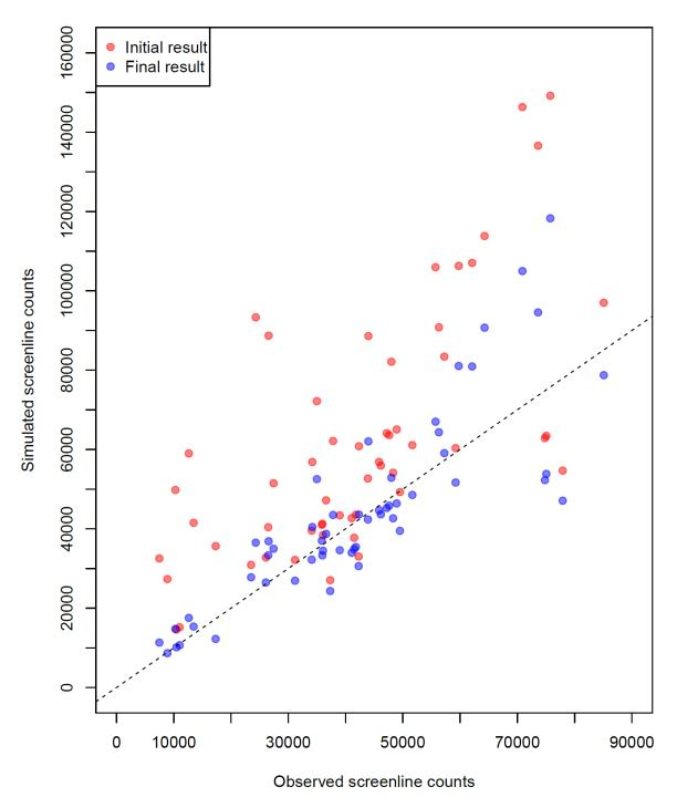
Fig. 10 Observed and simulated traffic count of each screenline.
