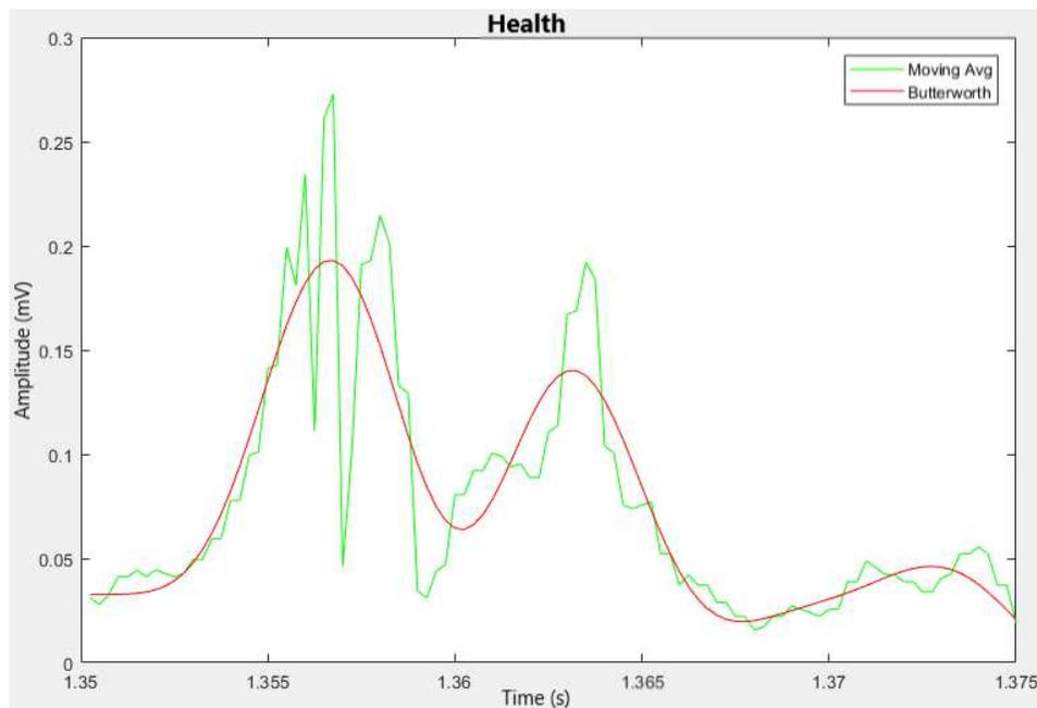
Figure 4. Step to find the linear envelope of signal
