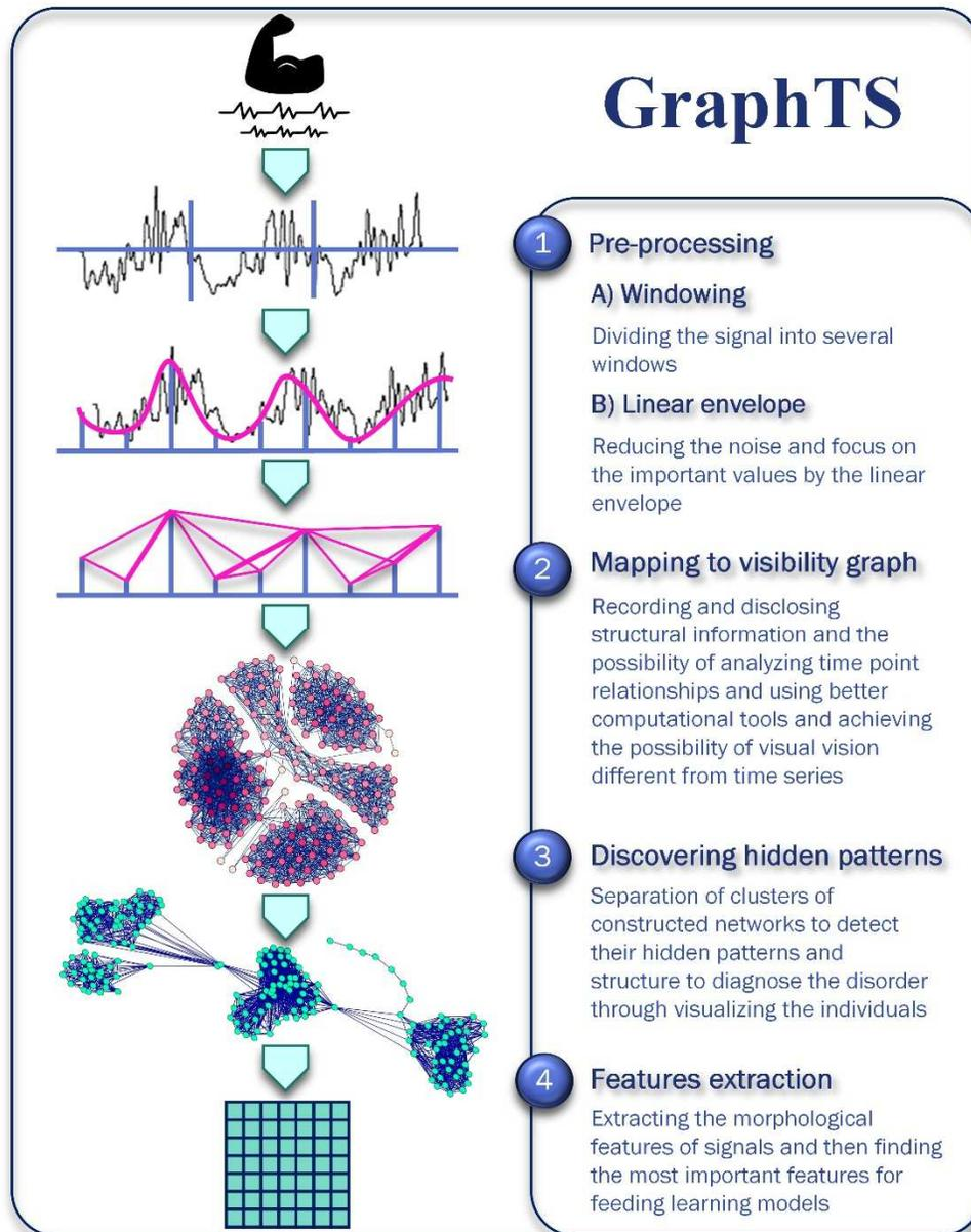
Figure 2. The overall process for the proposed GraphTS method
