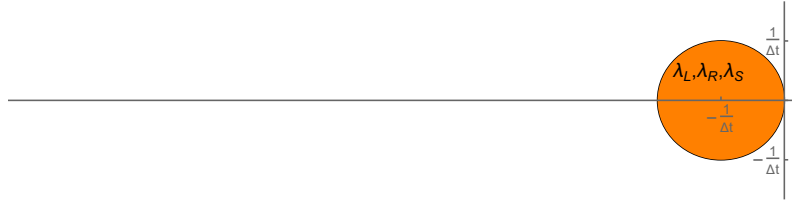
(a) Stability region of Forward Euler scheme (FE). The whole domain uses one time step \Delta t that determines the stability of all modes.
