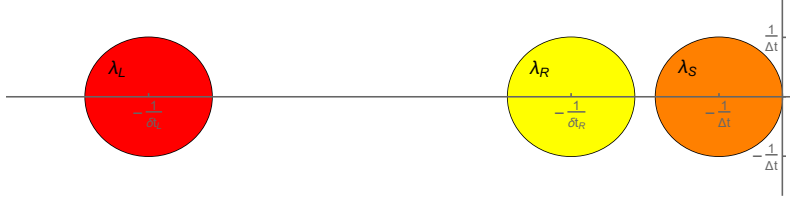
(c) Stability region of Adaptive Projective Projective Forward Euler scheme (APPFE). Both the stiff domain and the non-stiff domain each use one inner time step \delta t_{L,R} for fast modes and one time step \Delta t for the other modes.
