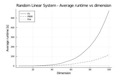
Figure 4: Average running time (over 10 iterations) of the FS (solid line), PBSR (dashed line) and Exponential (dotted line) algorithms applied to random linear systems of dimension  $5, 10, \ldots, 100$ .
